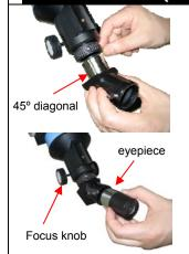
**Insert 45º diagonal:** Insert the diagonal into the eyepiece side of the telescope. Tighten the thumbscrews to a firm feel only.
